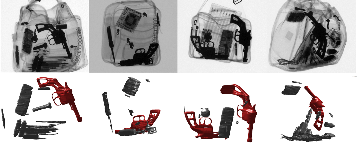
Fig. 9: Example of 3D reconstruction of the segmented objects in different travel-bags. In red we show the detected handguns after the matching and geometric consistency steps.
