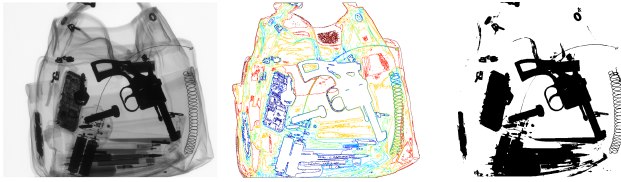
Fig. 7: Segmentation: original X-ray image, geodesic contours and binary image.
